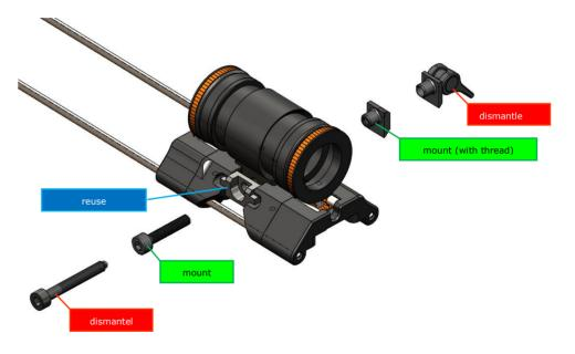
Put both plugs of the Anti-mirage strap holder in the drillings on the outside of the front sight base. Screw the both with the Anti-mirage strap holder to delivered screws on the inside. Balance bolts cannot be used together with the Anti-mirage strap holder.
